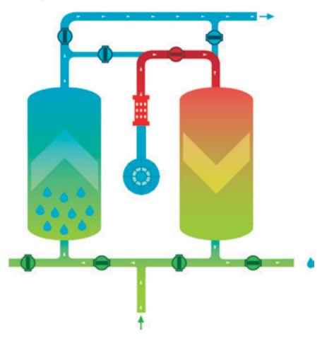
After heating, the desiccant beads need to cool down before they can start adsorbing again. The cooling can be done with dry compressed air, with cold ambient air or with cold compressed air. Each cooling method has its benefits and backdrafts.
